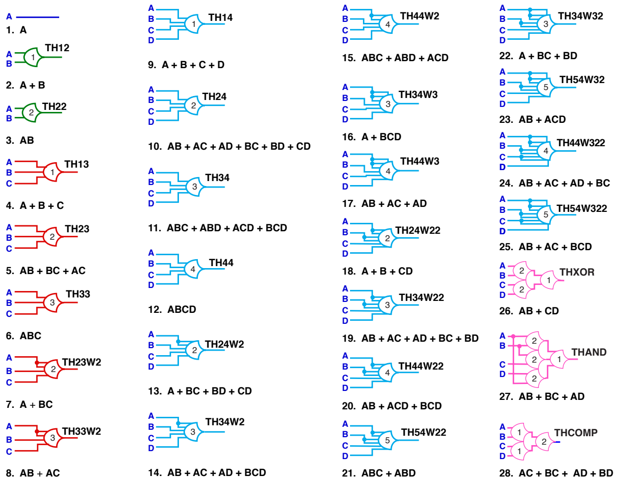
Figure A.2. The 28 NCL library operators with their corresponding positive Boolean functions.
