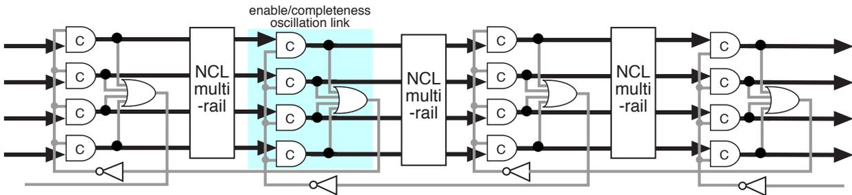
The entire flow path can be rendered solely in terms of C elements and OR gates; DIMS essentially. Or the identical functionality can be rendered several times more efficiently in terms of the more general NCL.
