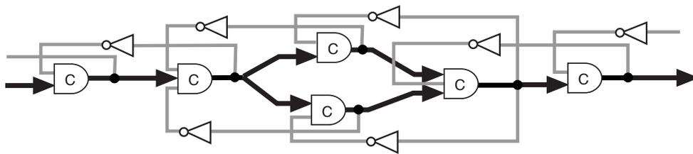
Arbitrarily complex networks of linked ring oscillators can be formed with conditional links. It is a spontaneously flowing network of linked ring oscillators that replaces the single ring oscillator of the clock.
