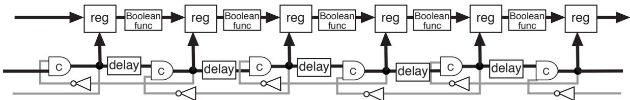
One wavefront value A can be assigned to mean data and the other value B can be assigned to mean “not data” (spacer, null) and the combinational computations can be designed with a delay insensitive encoding such as dual-rail employing completeness detecting registers to determine the completeness of computation. In this case the flow path of the oscillation passes through the computation and the registers. The oscillations implement the handshake protocols with the registers.
