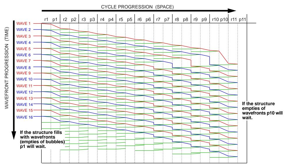
If p1 is slower than p10 wavefronts flow out of the structure. If p1 is faster than p10 wavefronts flow into the structure.
