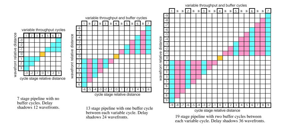
The slow delay in the center (gold) projects its wavefront shadow right and up and its bubble shadow left and down.
