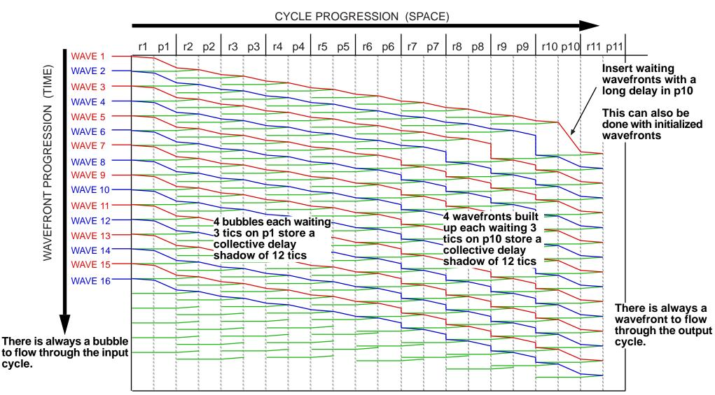
As long as cycles p1 and p10 cycle periods are equal there will always be 4 wavefronts between p1 and p10.
